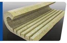
MinWool-1200® Field-Formed Pipe insulation is a water-repellent, factory v-grooved mineral wool board with a unique contact adhesive in the grooves. It is manufactured to specific pipe sizes with a variety of facing options. MinWool-1200 Field-Formed Pipe ships flat and allows for easy forming at the job site.
