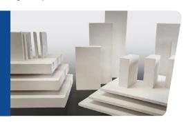
Super Firetemp® boards are inorganic, high-temperature boards with exceptional strength and insulating qualities, produced in various densities. Super Firetemp boards are suitable for fire protection applications, refractory backup, and can be machined into component parts of many shapes and sizes.
