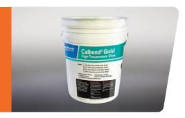
CalBond® Gold is a modified, silicate-based glue for thermal insulations. It sets quickly to provide a high-temperature bond for porous insulating materials. CalBond Gold is useful for bonding sections of calcium silicate or perlite high-temperature pipe or block insulation and to make mitered elbows, large insulating sections or other special shapes.
