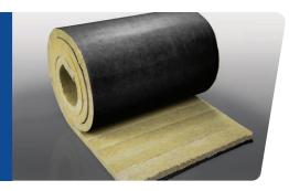
MinWool-1200® Lamella Tank Wrap is a water-repellent, lightweight, strong, flexible mineral wool wrap insulation with perpendicular oriented fibers. This insulation is produced to fit large diameter pipes, ducts, tanks and equipment, operating at temperatures from below ambient up to 1000°F continuous maximum service temperature.
