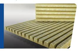
MinWool-1200® Precision Cut (PC) pipe insulation is a waterrepellent, factory v-grooved mineral wool board, manufactured to specific pipe or vessel sizes. It is offered with a variety of facings and is shipped flat in 4 mil plastic, allowing for easy forming on the job site.
