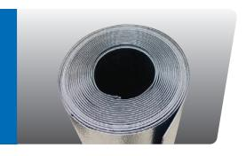
JM's 1 lb Muffl-Jac® sound barrier jacketing is a special high density, composite film laminated to 0.020" aluminum using a viscoelastic film adhesive. It simultaneously absorbs, dampens, blocks and isolates sound, and reduces noise levels radiated by piping and equipment.
